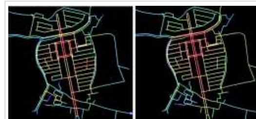
Figure 17. Axial map of R3 local integration zone 7 (left) and global integration Rn (right)
