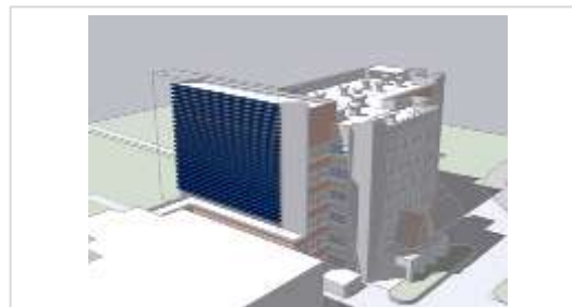
Figure 13. PV simulation on West facade 0.8 m
