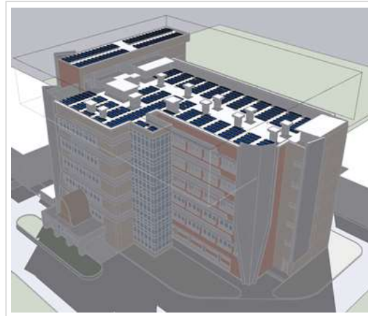
Figure 20. PV simulation on roof facing Nort 1 m
