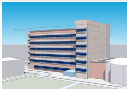
Figure 11. PV simulation on North facade 0.8 m
