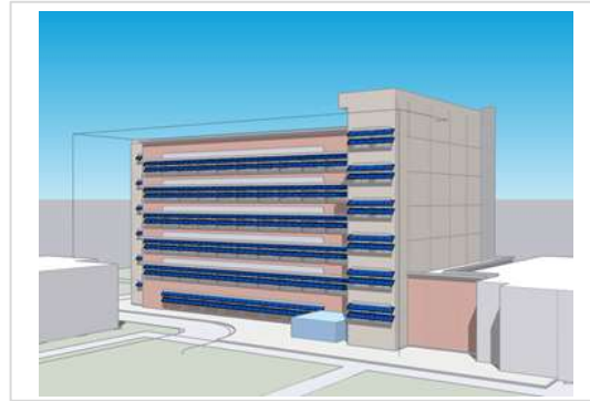
Figure 12. PV simulation on North facade 1 m
