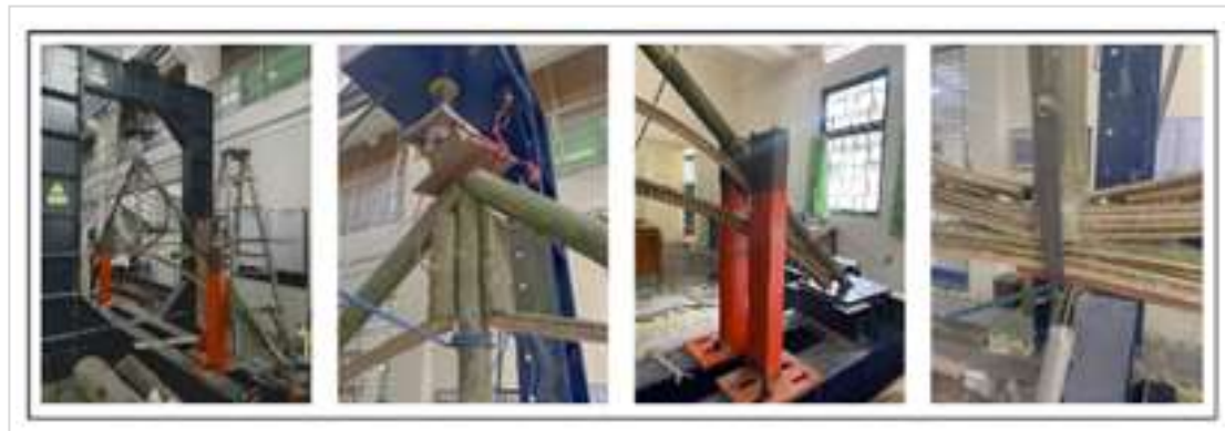
Figure 14. Experimental set up for bamboo truss compression testing using hydraulic press
