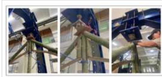
Figure 22. Test examination of peak performance in bamboo trusses
