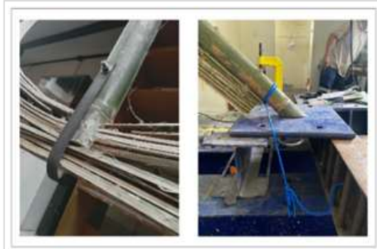
Figure 15. Experimental set up for bamboo truss compression testing using hydraulic pressure
