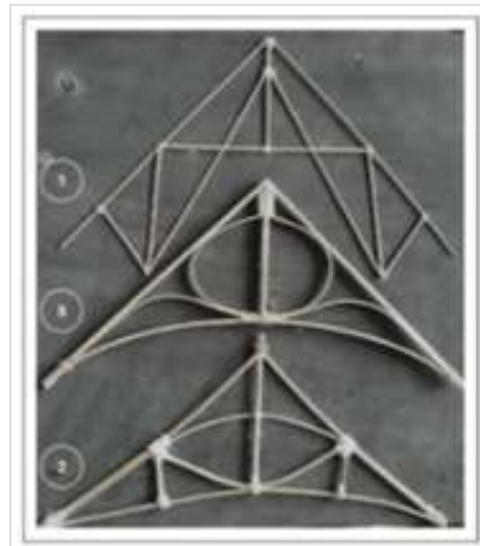
Figure 3. Evaluation of truss design stability
