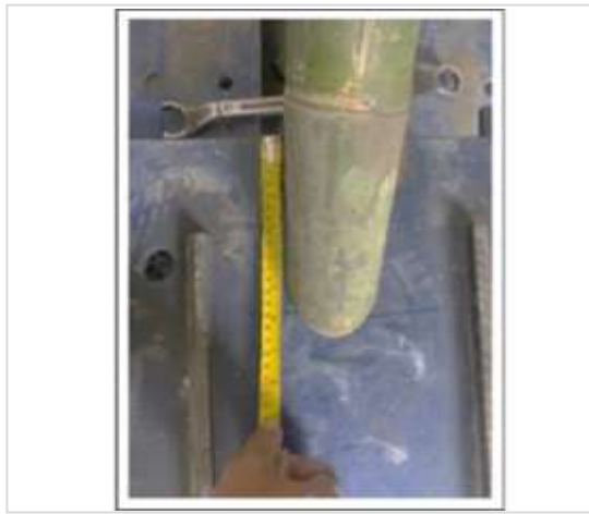
Figure 23. Shift of support (roll joint) after test
