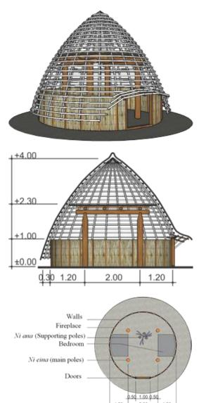
Figure 5. The plan and appearance of the *ume kbubu*
