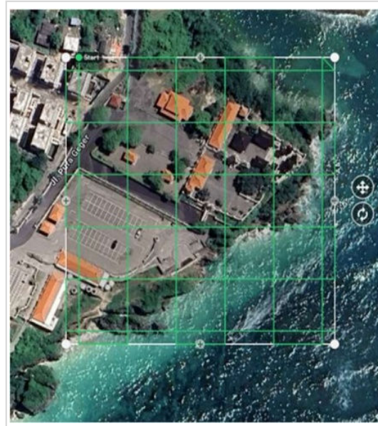
Figure 4. Example of image data collection stages using UAV/high resolution camera on temple area objects
